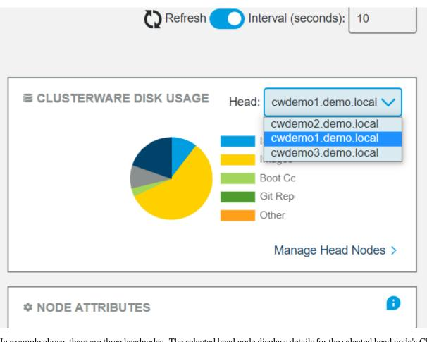
In example above, there are three headnodes. The selected head node displays details for the selected head node's ClusterWare disk usages for each of the various types of ClusterWare entities: ISOs, PXEboot images, boot configurations, Git repositories, "other", influxdb data, and the etcd database.
