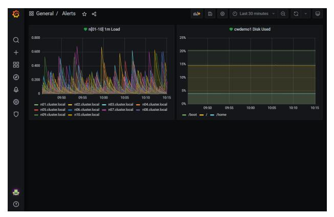
The first panel displays the CPU load levels for the first 10 compute nodes. The second panel displays the disk usage for one head node.
